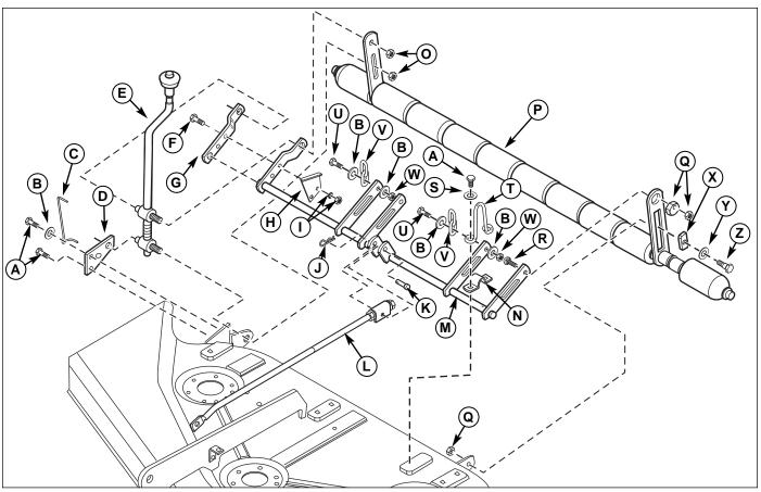
Figure 3. Installation 44" Rollers
